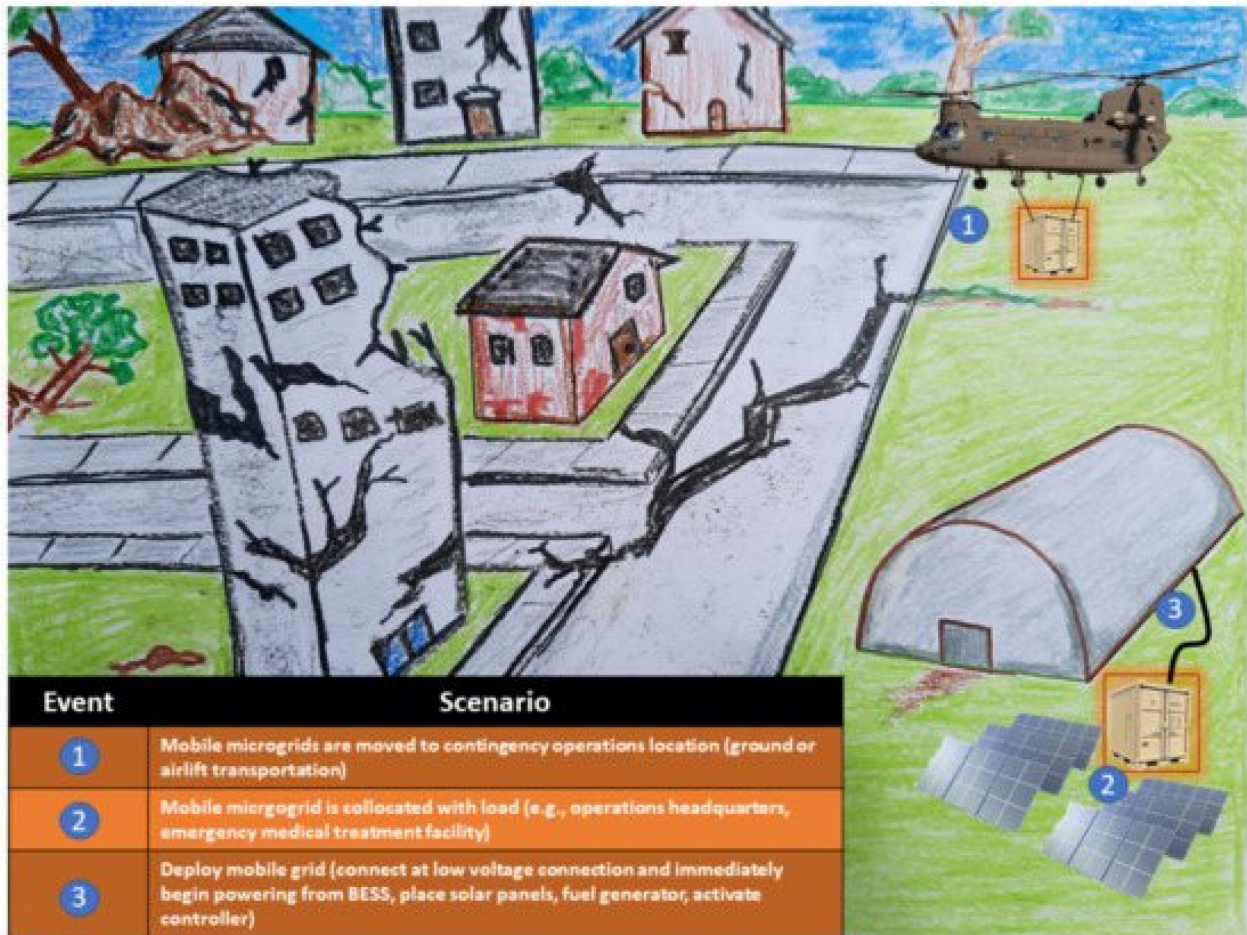
Figure B-5: Mobile Microgrid is Airlifted to Contingency Operations Location and can be Powered There. Used with permission of Douglas VanBossuyt, Naval Postgraduate School. Graphic originally published in: Varley et al., 2022. “Feasibility Analysis of a Mobile Microgrid Design to Support DoD Energy Resilience Goals.” Systems 10, no. 3: 74. https://doi.org/10.3390/systems10030074 .
